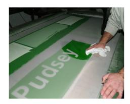
Activator is applied for capillary action to take effect
