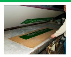
The stencil is left to air dry or by using a cool fan
