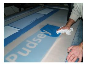
Activator is applied for capillary action to take effect
